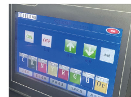
LCD monitoring screen, to detect the stability of the ink system and stepping system at any time, easy to operate and adjust
