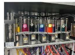
Ink negative pressure system, better ink fluency, ensuring stable output for high-speed production
