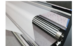
Felt roller to ensure smoother paper feeding
